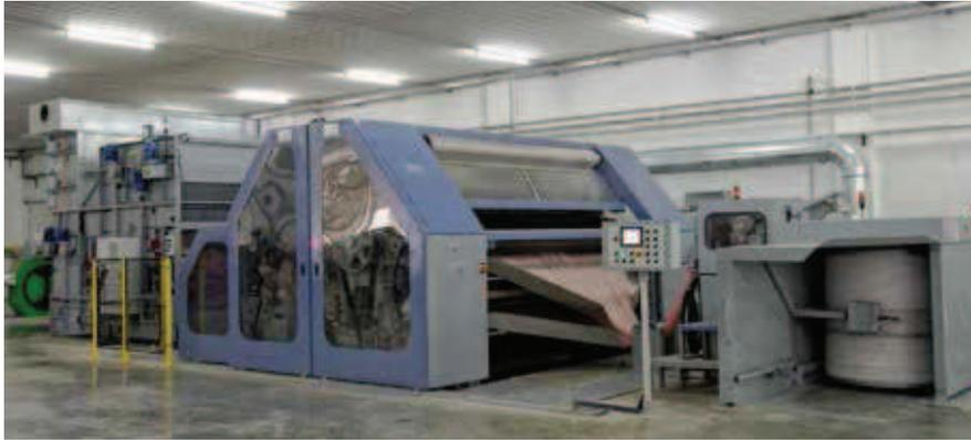
The drive control provides for a speed adjustable from desk control.
